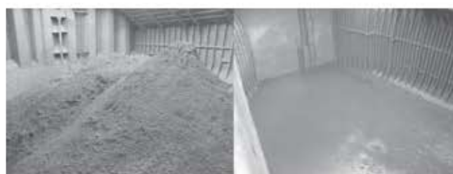
Iron ore fines before and after liquefaction.
